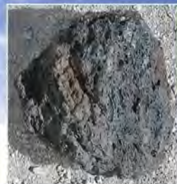
After TIFI treatment, slag is more friable, weaker and more porous.
